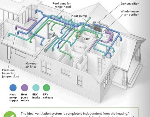
cooling system. Ventilation supply air is ducted directly to the bedrooms and living spaces while the ventilation exhaust air is drawn directly from bath-**GET IT** rooms, mudrooms, and other sources of moisture. By decoupling the ventila-RIGHT tion system, it can run regardless of whether the heating system is on or off. Additionally, balancing and commissioning the system to provide the correct airflows is much easier. -J.G.
