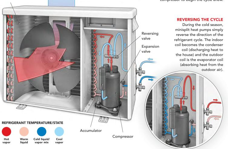
outdoor units, with one fan and one coil in each and refrigerant lines running between.
